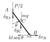
$$\begin{aligned} y_A &= l\cos\theta & \Rightarrow & \delta y_A &= -l\sin\theta\delta\theta \\ x_B &= l\sin\theta & \Rightarrow & \delta x_B &= l\cos\theta\delta\theta \\ y_C &= (l/2)\cos\theta & \Rightarrow & \delta y_C &= -(l/2)\sin\theta\delta\theta \end{aligned}$$
