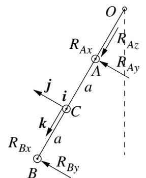
$$\mathbf{M}_C = \frac{d}{dt}(\mathbf{I}_C \cdot \boldsymbol{\Omega}) = \mathbf{I}_C \cdot \left[ \frac{d}{dt} \boldsymbol{\Omega} \right]_{\text{rel}} + \boldsymbol{\Omega}_{\text{ref}} \cdot (\mathbf{I}_C \cdot \boldsymbol{\Omega}), \quad (1)$$
